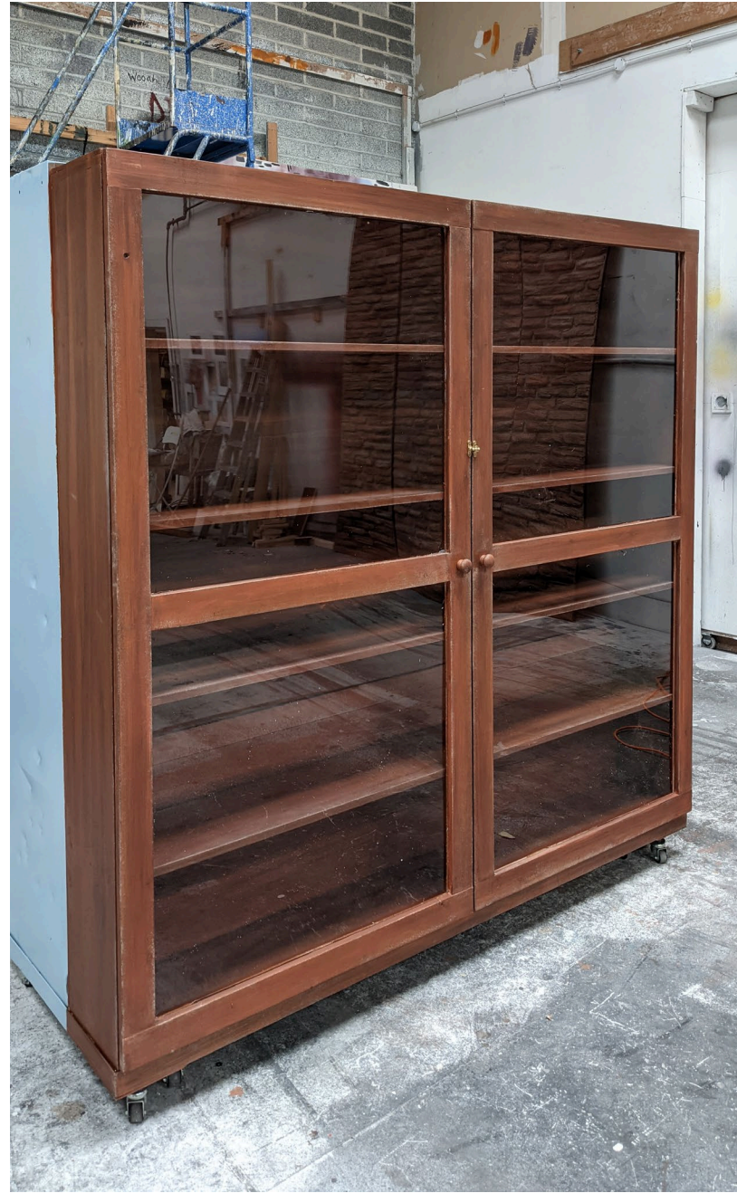
Creating a wood grain effect for the shelves and benches using washes and glaze, with rollers to age and finish.
