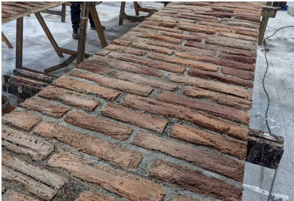
Brick walls – Carved polystyrene stuck on panels using latex adhesive in roman brickwork fashion. This was then textured with Idenden and Artex, then painted in multiple layers of washes and spatters.
