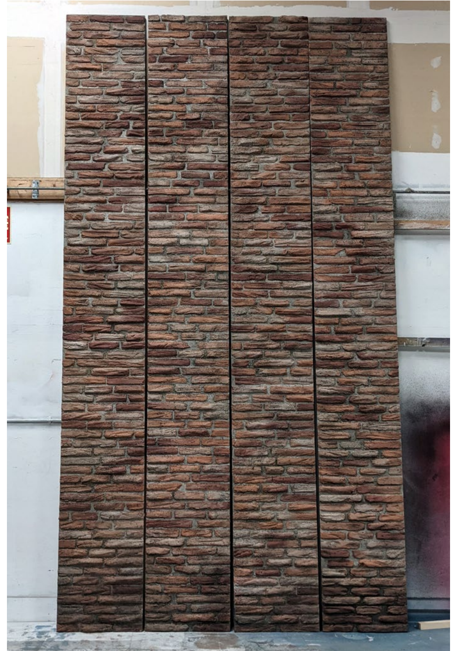
Brick walls – Carved polystyrene stuck on panels using latex adhesive in roman brickwork fashion. This was then textured with Idenden and Artex, then painted in multiple layers of washes and spatters.
